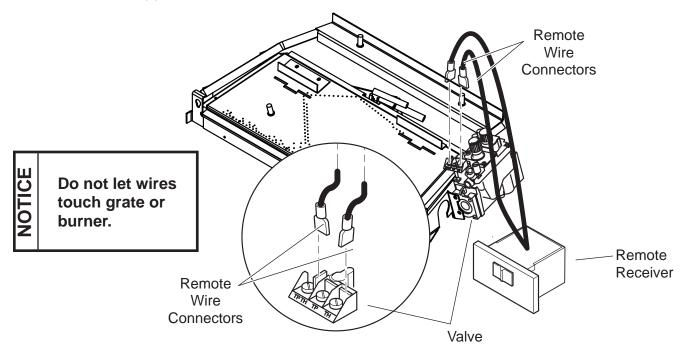
Figure 18 - Installing Remote Receiver
